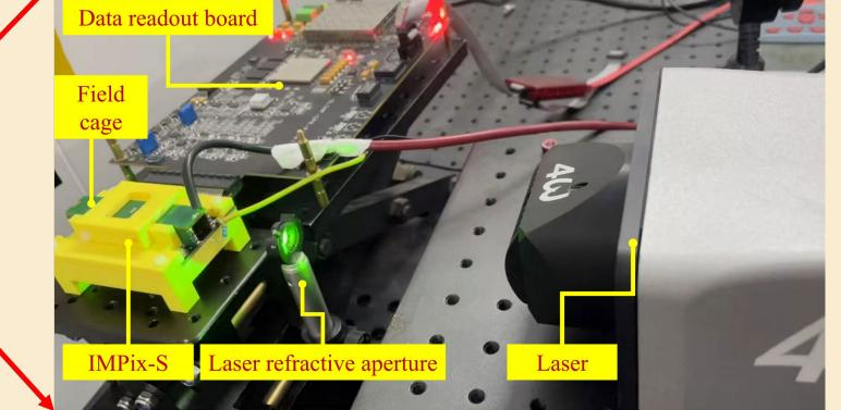
The IMPix-S chip comparator has a threshold of 2 ke<sup>-</sup> and operates in continuous scan readout mode with a scan frequency of 10 MHz. The high voltage case provides 1500 V high voltage to the field cage.
