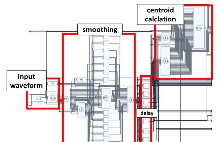
The signal-to-noise ratio is important to obtain high time resolution.For denominator, the white-noise component is cancelled by simple integration. On the other hand, we have to consider the error propagation of the numerator g.
