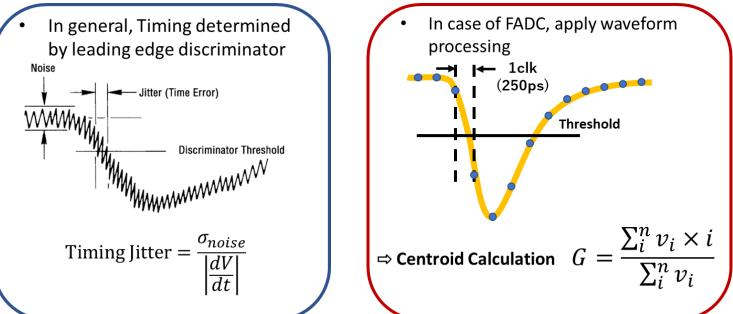
Here, Centroid Calculation was adopted. The centroid calculation is independent of the slope form and can be applied to any waveforms. Furthermore, in this equation, G is timing, and the denominator is charge, so time and charge information can be obtained simultaneously.
