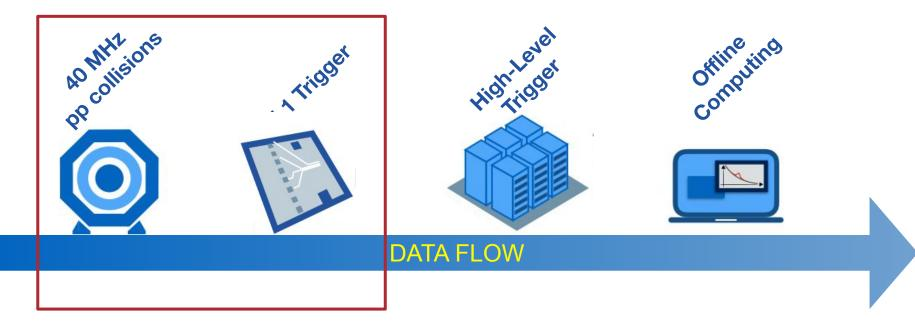
ML in trigger and sensor applications must be implemented in FPGAs or custom ASICs! Must be robust to noise and radiation and meet high throughput low latency requirements.
