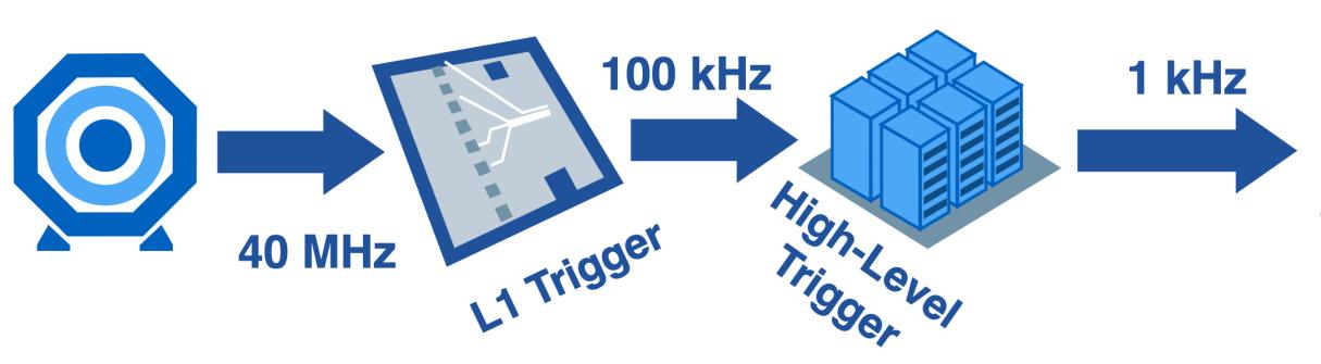
Trigger algorithms become progressively more complex. The latency requirements decrease at each subsequent level.
