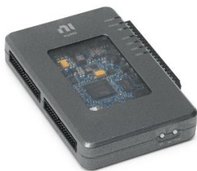
Figure 1. Hardware illustration of the NI MyRIO device, featuring an FPGA, ARM Cortex-A9 processor, analog input (AI), and digital input and output (DIO) [4].
