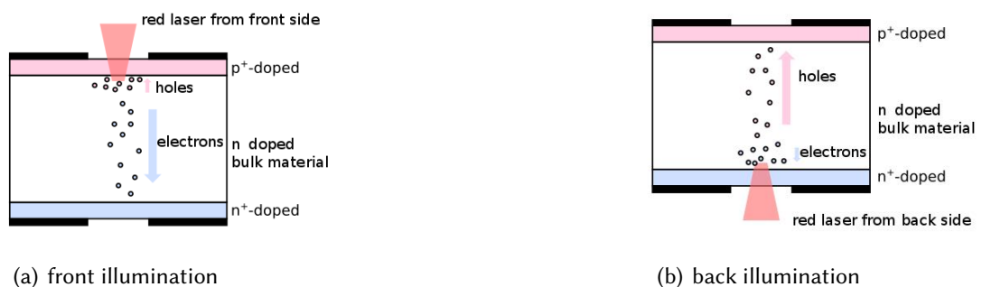
Figure 3: TCT measurement illustrating the two illumination methods and the corresponding charge movement in the sensor bulk.
