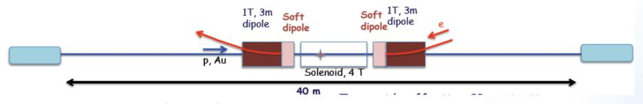
Use soft (~0.05 T) bend for final bending of e beam to IP, to shield detector from all but the very softest synchrotron radiation
