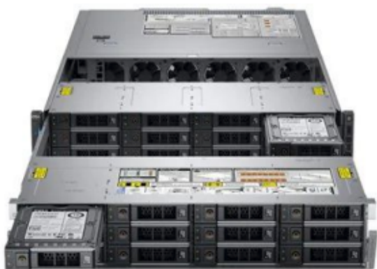
Figure 1. Image of the new Dell R740xd2, 2U rack systems with 24 drive density (12 front and 12 mid-plane all hot swappable). Other specifications include: 2 x Intel Xeon Gold 5218 2.3G, 16C processors; 12 x 32GB RDIMM 2666MT memory; 24 x 14TB 7.2K RPM SATA 6Gbps drives; Intel XXV710 Dual Port 10/25GbE network.
