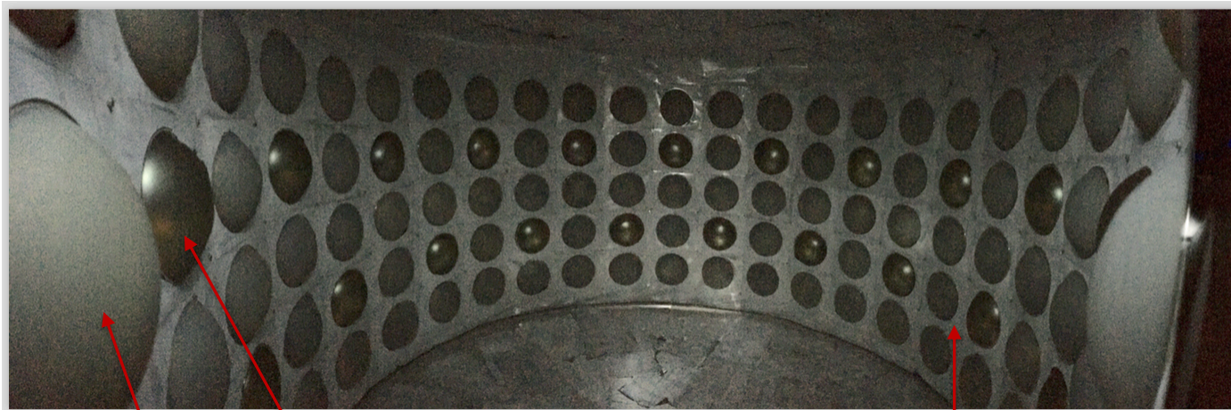
TPB coated PMTs Uncoated PMTs
