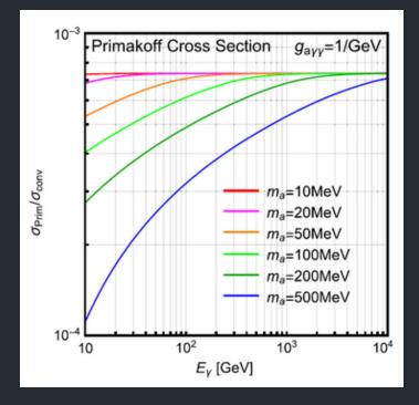
Ratio between the Primakoff and pair-production cross section (in iron)
