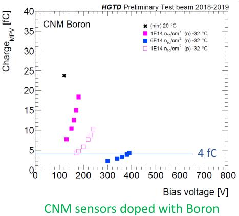
Charge computed as the integral of signal waveform divided by sensor transimpedance
