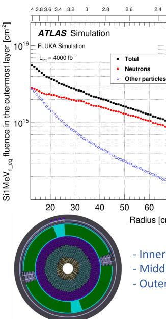
With FLUKA simulation, radiation level expected at R =12 cm: fluence >  $5.6 \times 10^{15} n_{eq}/cm^2$ total ionizing dose ~ 3.3 MGy
