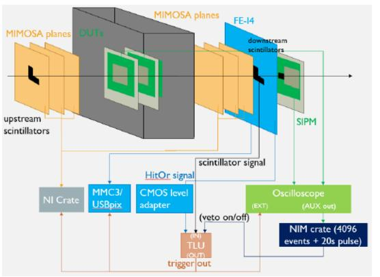
Oscilloscope needs time to empty the buffer At CERN beam has a spill-structure (~ 4 s-long, every 16 s) At DESY, continuous beam ⇔ busy signal implemented to simulate a spill-like beam (20 s paused)
