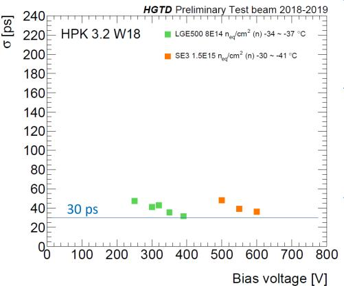
HPK sensors doped with Boron and irradiated with neutrons
