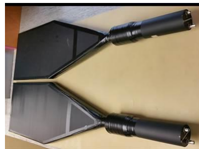
Beam Trigger (2 pairs of scintillators)
