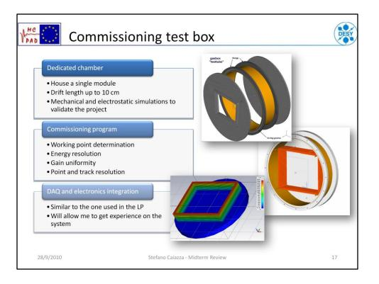
To commission the LP module before using it in a test beam campaign on the LP itself we decided to use a dedicated chamber. I'm in charge of the designing and producing of this chamber as well. The design is such to house a single LP module in a drift chamber up to 10 cm long. I performed electrostatic and mechanic simulations during the design phase to validate the project. I kept the design as modular as open as possible to be able to adapt the system to new requirements.
