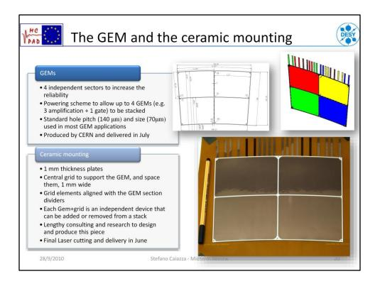
Because a GEM is like big capacitor, to avoid destructive discharges it's necessary to reduce the amount of energy that can be released in each of these discharges. For this reason the GEM surface has been divided in 4 electrically independent sector, each of which as an area about the same as a standard 10X10 cm<sup>2</sup> GEMs, usually used for testing.
