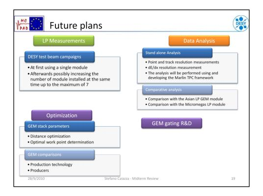
Another of the main goals of the commissioning phase will be the optimization of the GEM stack, which means optimizing the parameters of the GEM stack, e.g. distance between the GEM and voltage loads across the GEM and the gaps In a second moment it may be possible to compare different GEM types and producers in this same test box comparing, for example, the single mask etched GEMs with the normal double mask etched GEMs, or different producers like CERN, Techetch, SciEnergy ...
