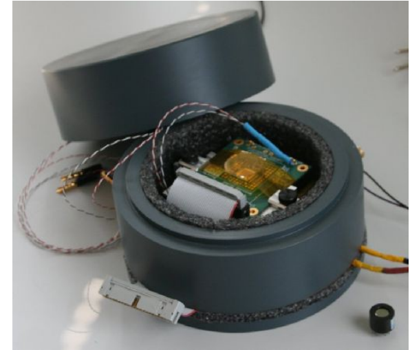
Cold box for testing irradiated samples
