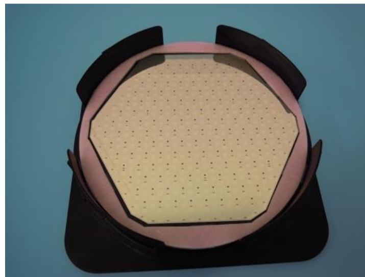
8-inch silicon sensor (low-density)
