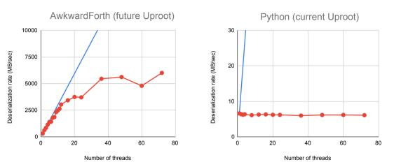
AwkwardForth machines are lightweight: we can make one per thread. Python is inhibited by the GIL. Scales linearly up to RAM access ceiling (5 GB/sec).
