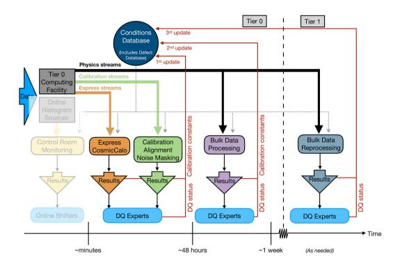
used in parallel with *online* chain which provides immediate (but limited) feedback in the control room; offline DQM allows comprehensive study of all recorded data
