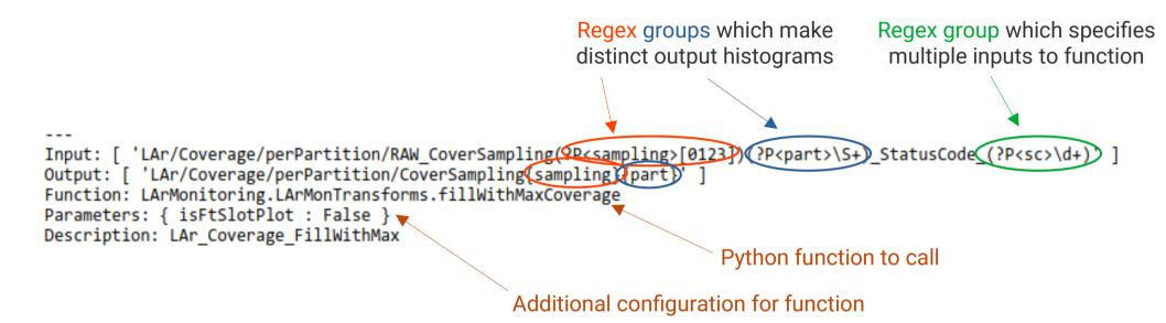
Same YAML configuration & user code used for offline and online applications; only difference is I/O plugins
