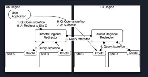
XRootD protocol enables high performance, scalable fault-tolerant access to data repositories of various kinds, including EOS.
