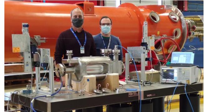
Bead-pull measurements at FNAL on AUP Prototype #1 (Sept 2020)
