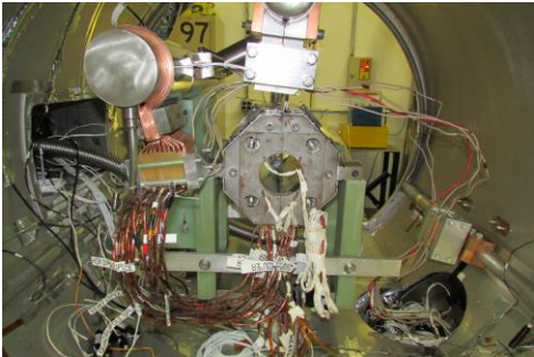
Conduction cooling test
