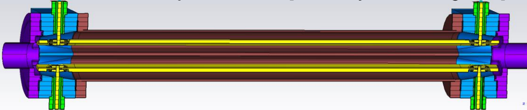
Cross section of injection kicker [Courtesy of M. Sangroula]
