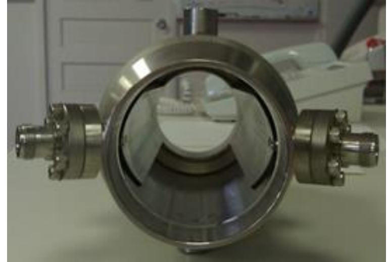
Existing stripline BPM (above) will be shielded; button BPMs (below) will be installed adjacent
