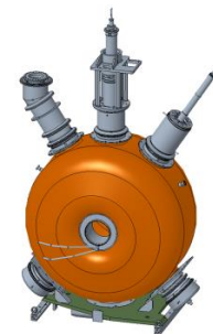
Hadron - 197 MHz bunch compression cavity
