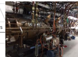
Hadron – 24.5 MHz acceleration cavity
