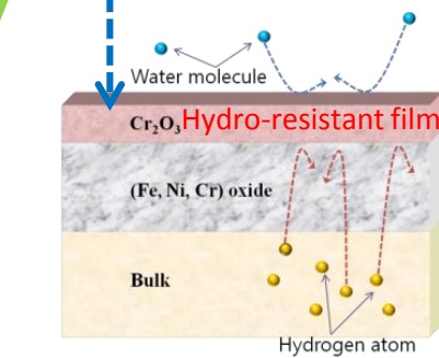
Hydrogen barrier by the Cr_2O_3 layer
