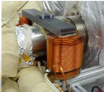
Steel laminated core magnet installed in RHIC
