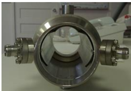
Existing strip line BPM will be shielded
