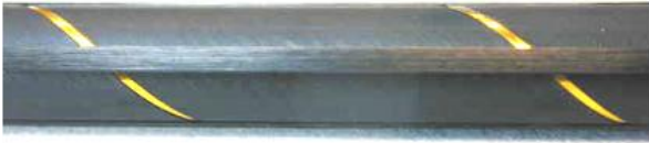
Two 9.5mm wide strips of coated polyimide film spirally wound back-to-back with a 50 \pm 10\% overlap
