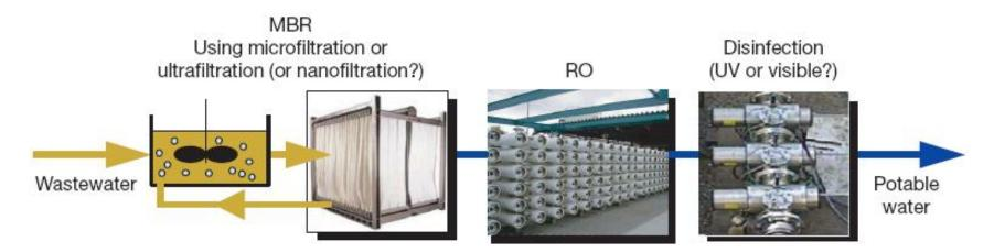
Next generation membrane treatment system for direct conversion to potable water. M. Whitby, and N. Quirke, Nat. Nanotechnol. **2**, 87 (2007).
