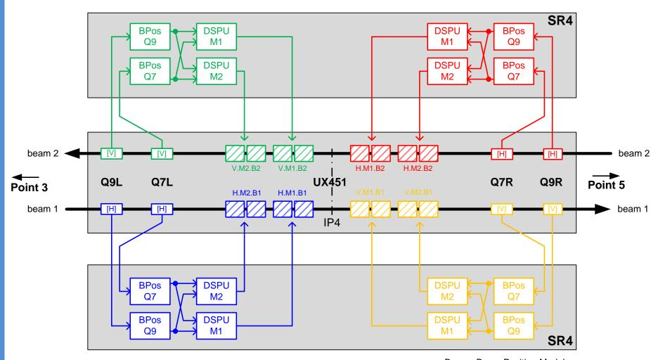
Bpos – Beam Position Module DSPU – Digital Signal Processing Unit
