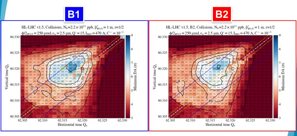
Slight DA reduction with anti-telescope (although lower octupoles).
