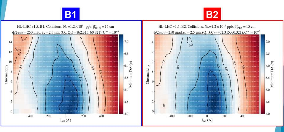
For optimized working point (B1, EOL, negative octupoles, DA<sub>min</sub>=6.21 σ).
