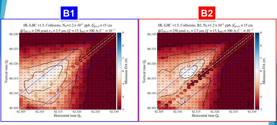
1 working point for B2, marginal for B1 (without IP1-IP5 phase advance optimizations).
