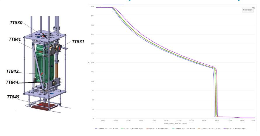
With the cooling of the thermal screen, the temperature inside the cryostat dropped to 130K and the temperature gradient along the cavity was less than 10K during the process. Since T <130K, we asked the cryogenic team to cool down quickly.
