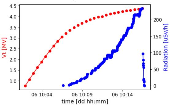
No field emission were observed below  $\sim 3.5 MV$  At 4.1 MV:  $\sim 85 \ \mu Sv/h$
