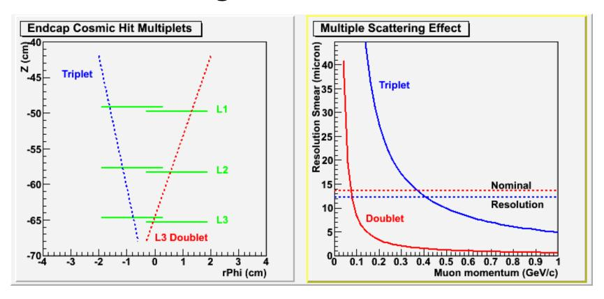
Pin a straight line on hits from inner most and outer most hits (L1,L3 in the picture but really L0,L2) and extrapolate line to middle layer to look for residual. Triplet residual is sqrt(3/2)\*single hit resolution. Doublet sqrt(2)\*single hit.
