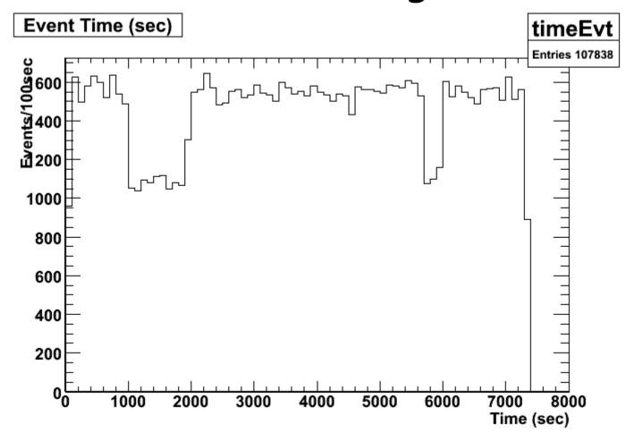
~15 Hz trigger rate is close to expectation if allowing some noise triggers.
