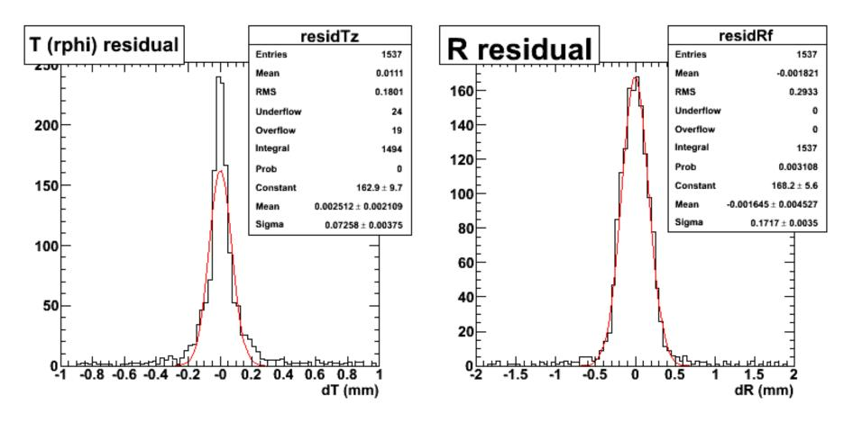
$r\phi$  residuals down to ~73  $\mu m$  (or better in the core) (still ideal geometry !) and the remaining may be really alignment issues
