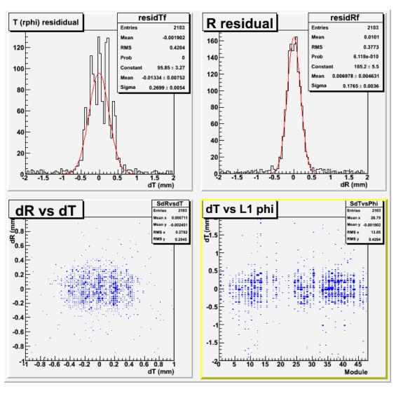
Getting much better and radial resolution of ~180µm already approaching intrinsic resolution, with just the ideal geometry!
