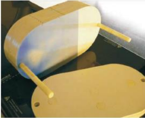
Figure 3.6 QUASIMODO CarPet phantom with Gafchromic EBT film after the delivery of a 5-arc IMAT treatment of an elongated tumour adjacent to the thorax wall.
