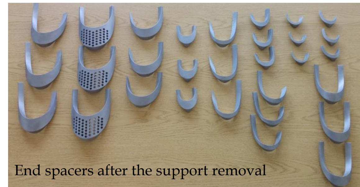
End spacers after the SLM process
