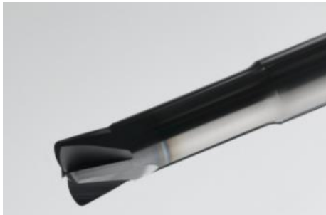
High feed mills for roughing Ø2 mm, 45k rpm, 0.06 plunge
