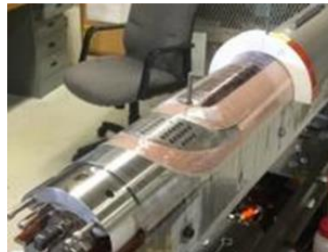
End spacers during coil assembly at FNAL
