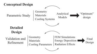
Figure 1: Diagram of the design phases for the Linac4 Main Dump.
