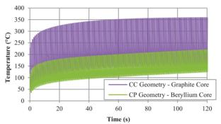
Figure 5: Peak temperature evolution in the CC geometry with graphite core and in the CP geometry with beryllium core.
