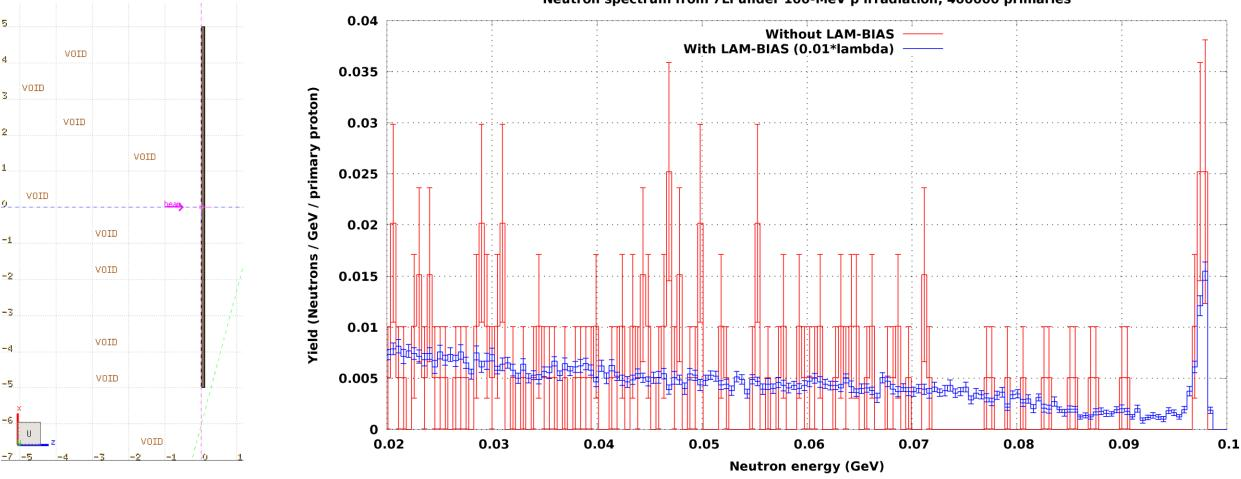
Neutron spectrum from 7Li under 100-MeV p irradiation, 400000 primaries
