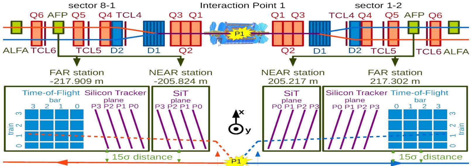
AFP consists of 4 Si pixel stations, 2 on each side of the interaction point at approximately 205 and 217 m.
