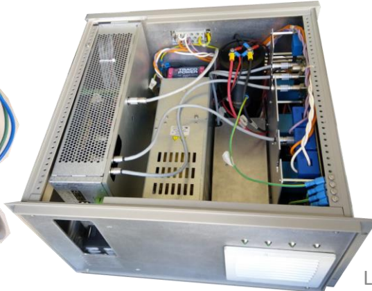
BWSIDC automated functional bench with scanner (Jonathan) Python based script using JTAG (soon IP-BUS)
