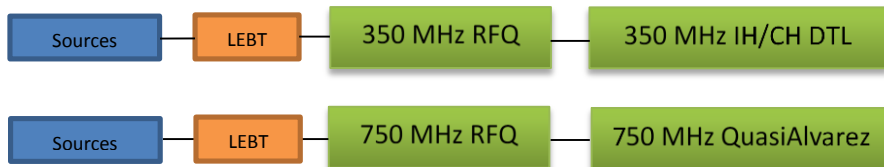
Two alternative concepts for a new 7 MeV injector linac at higher frequency ( q/m = 1/3 )
