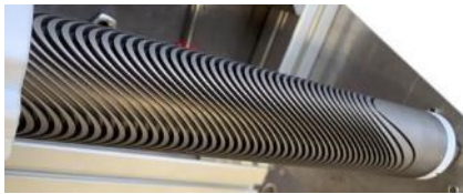
Solution for curved and straight CCT coils combining dipole and quadrupole in the same winding - Courtesy G. Kirby and J. van Nugteren, CERN
