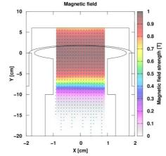
• Generating (single) charged particles and observing their behaviour (example: electrons correctly bent downwards by the dipole described above)
