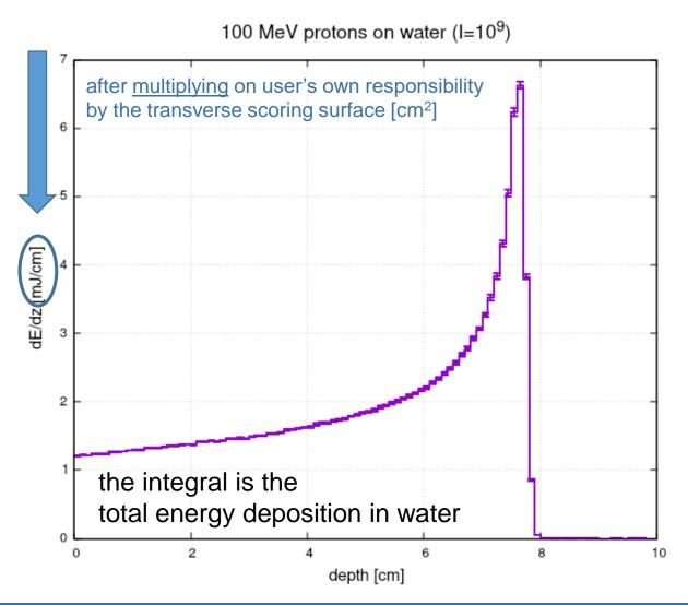
for each z-bin, the highest value 1D Max on the transverse scoring surface
