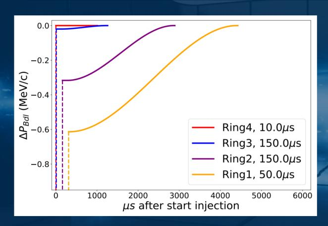
Special dipole "Bdl" trim circuits will offset the magnetic field at the start of injection to each ring
