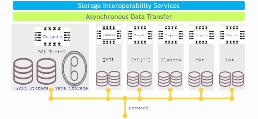
Storage endpoints of perhaps different QOS; data-exchange managed through WAN transfer protocols and orchestrated by storage interoperability and high level services.
