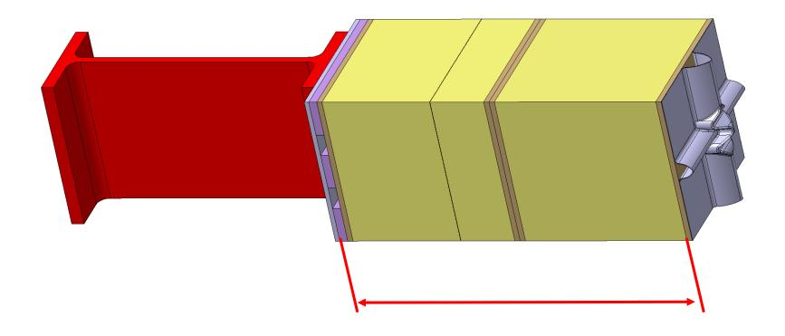
Replacing internal blocks with insulating panels 1200x600x100 mm
