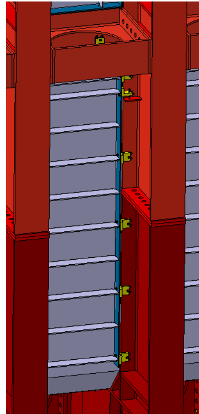
Clamps on bottom wall plate
