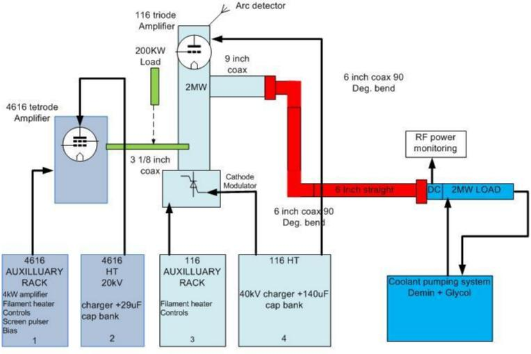
Daresbury test setup for proving amplifiers/power supplies
