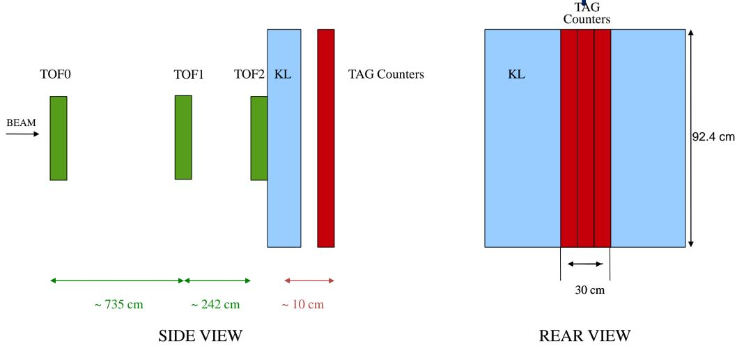
TAG Counters – 3 scintillator slabs, 10 cm wide each, 2.5 cm thick MICE CM27, July 2010
