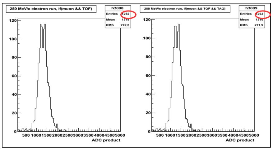
An example of electron run with momentum 250 MeV/c at the target. Estimated muon momentum through beam line tables at KL entrance ~ 165 MeV/c. Fraction of muons reached TAG counters ~ 98%.
