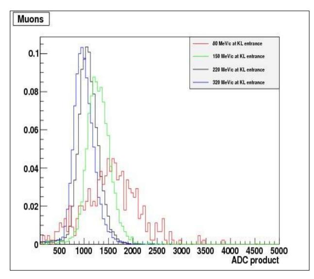
Muon dE/dx for Pb (the heaviest ingredient in KL) becomes smaller with momentum increasing.
