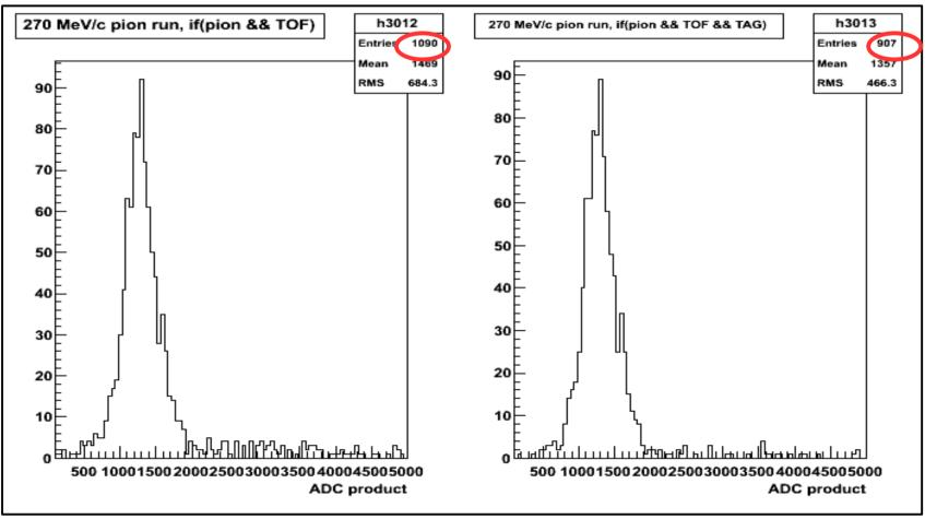
An example of pion with momentum 270 MeV/c at the target. Estimated pion momentum through beam line tables at KL entrance ~195 MeV/c. Fraction of pions reached TAG counters ~ 83%.
