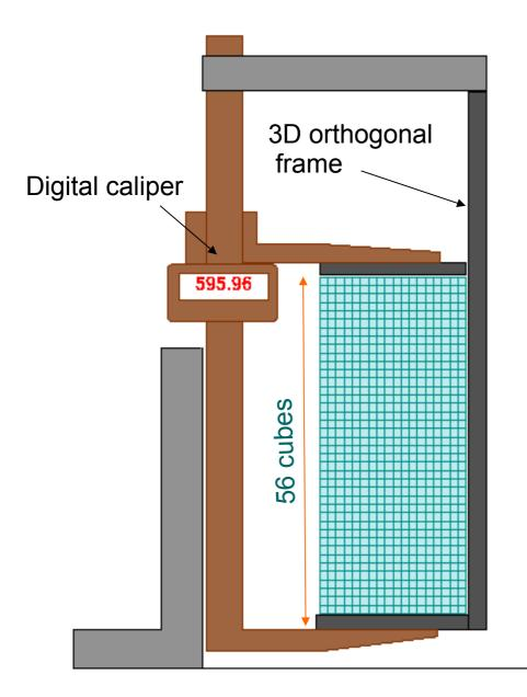
3D orthogonal frame with high geometrical accuracy was built of milled steel plates.
