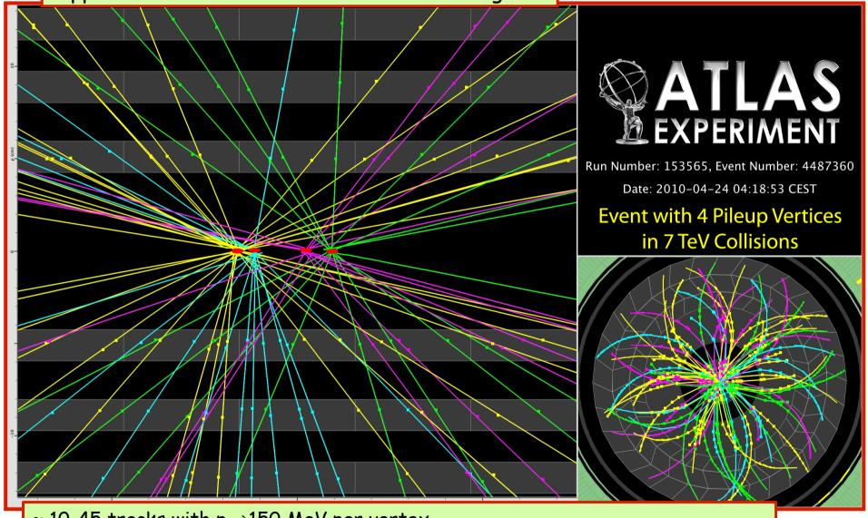
~ 10-45 tracks with  $p_T$  >150 MeV per vertex Vertex z-positions : -3.2, -2.3, 0.5, 1.9 cm (vertex resolution better than ~200  $\mu$ m) Expect handful of 4-vertex events in this run
