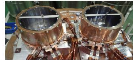
Fig. 11. Prototype coils on test facility
