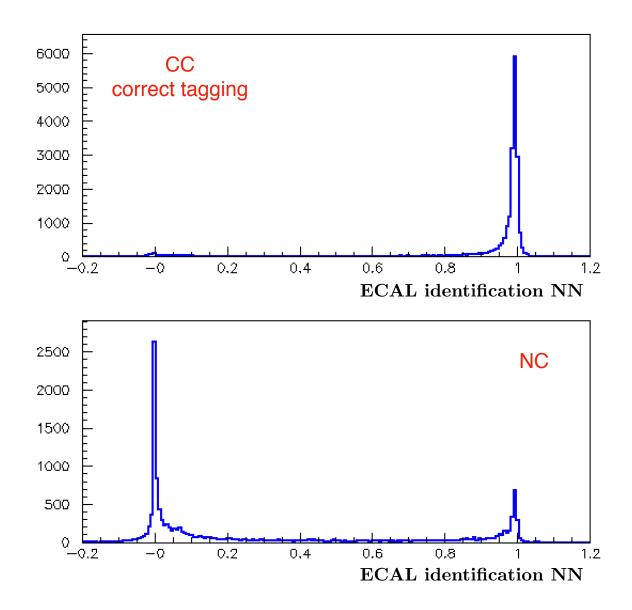
Tagged tracks reaching barrel ECAL and NOT reaching outer yoke
