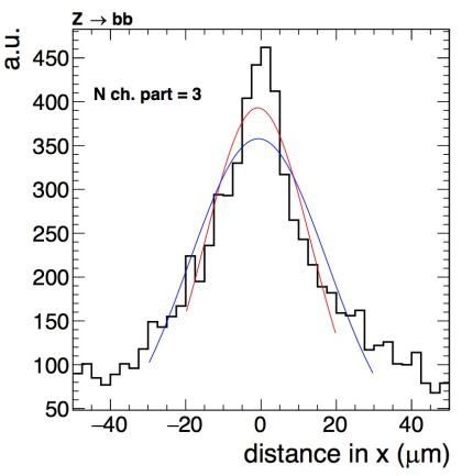
Example: decays with 3 tracks (charged particles) The distance in x to the closest reconstructed displaced vertex is shown
