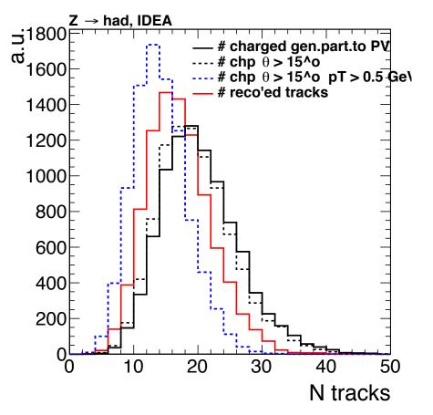
Comparing generated particles with different cuts and reconstructed ones
