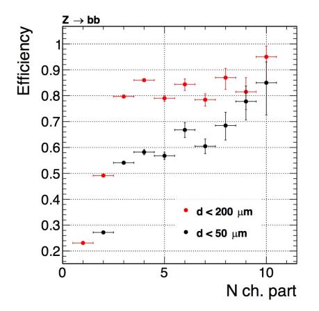
Efficiency that a gen-level displaced vertex (i.e. secondary/tertiary/etc from the B's) is matched with a reconstructed displaced vertex, within 200 μm or 50 μm
