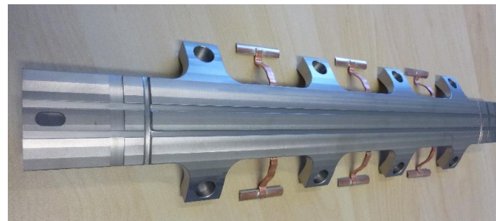
Tungsten absorber with 3 thermal links
