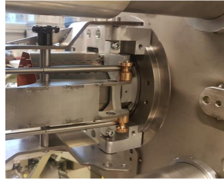
In-situ cooling tube bending
