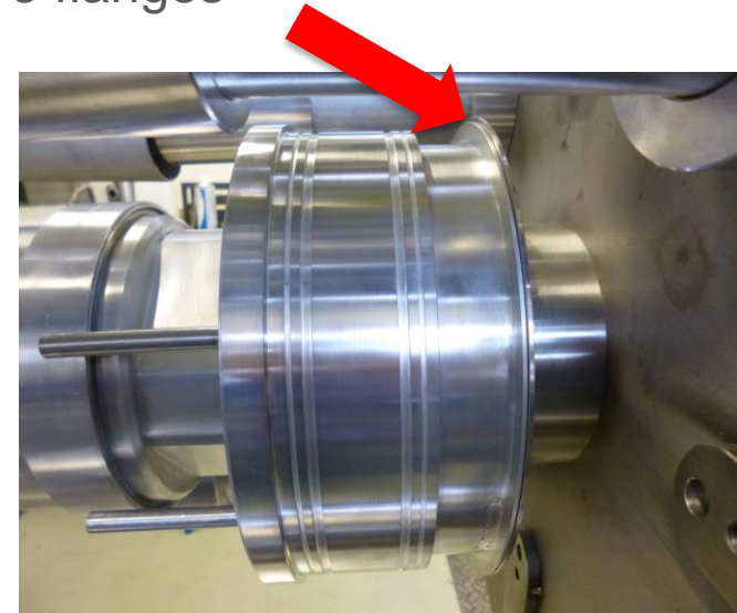
Installed end flange
