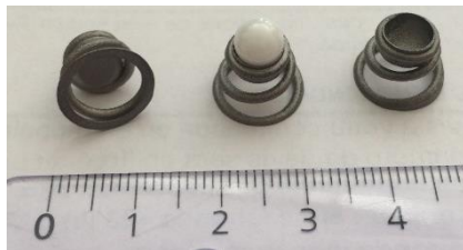
3D printed titanium spring with ZrO 2 ball
