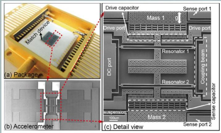
**Einstein Telescope:** MEMS accelerometers with novel **Cryogenic CMOS** signal conditioning integrated circuits (e.g. for low-temperature vibration control)
