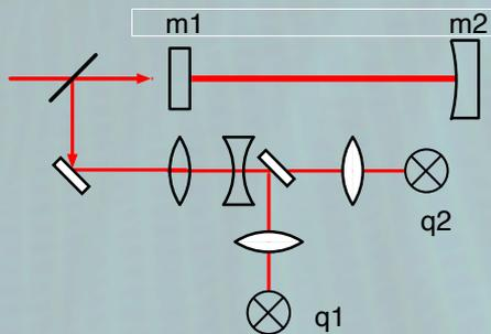
Optimal wavefront sensing scheme for Fabry-Perot cavity alignment
